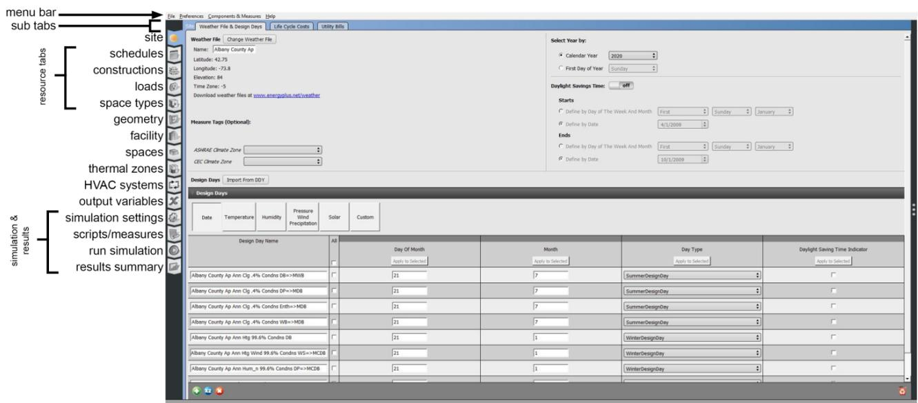
Figure 6. OpenStudio Construction Sets interface.
